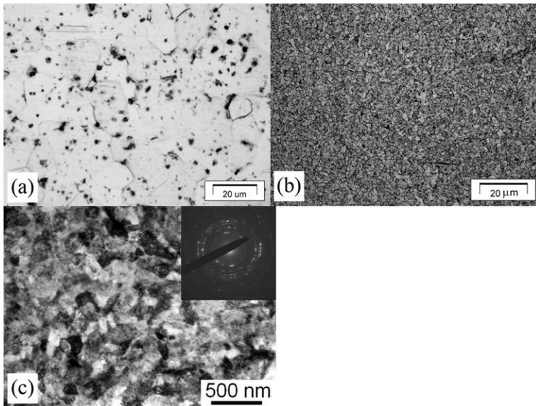
Fig. 2. Microstructure of Grade 4 CP Ti: (a) the initial coarse grained rod; (b) and (c) cross-section rod after ECAP-C + drawing (optical (a and b) and TEM (c) pictures).
