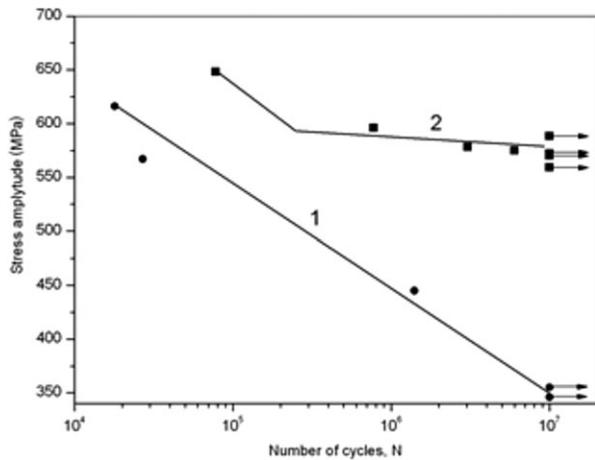
Fig. 3. Fatigue properties of Ti Grade 4 1 in the as-received condition, 2 after ECAP-C with drawing to 75%.
