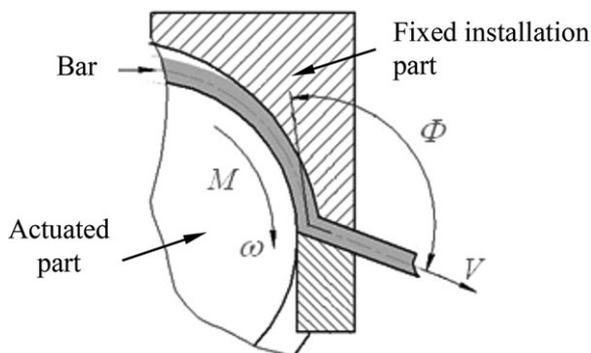
Fig. 1. The principle of ECAP-C technique.
