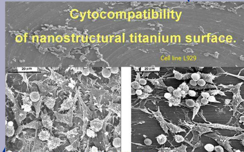
Fig. 3. Occupation of the mice fibroblast cells L929 after 24 hours: Nanostructured (left) and conventional (right) CP Grade 4 titanium.
