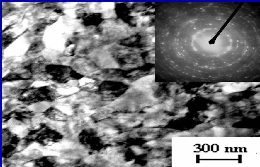
Ultrafine grain Grade 4 commercial purity titanium:
